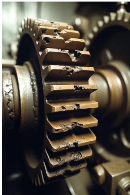
Figure 1 – Deep pitting cavities on bronze worm wheel teeth
